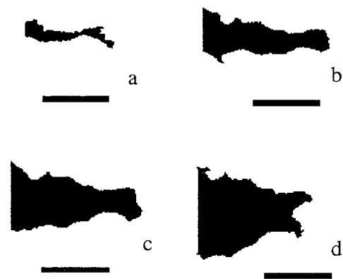
Figure 3 Cross-sectional shape of the crack tip of the AH (5 Torr H 2 ) sample for the following values of the stress intensity factor K_I (a) 15 MPa√m; (b) 22 MPa√m; (c) 25 MPa√m; (d) 30 MPa√m. In each case the scale bar has a length of 10 μm.
